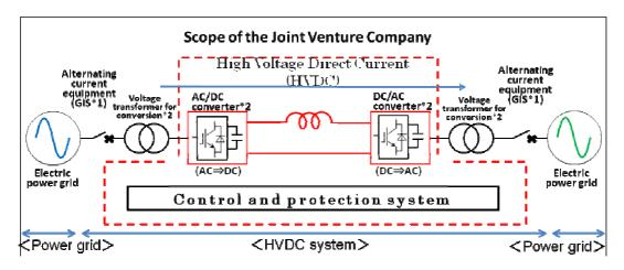
HVDC systems are used to transfer power between two electric power grids.
