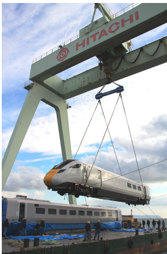
A Class 800 train is being loaded for shipment
