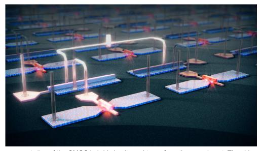
Artistic representation of the CMOS hybrid circuit used to perform the experiment: The chip contains two cells, each composed of one control transistor and one quantum device.
