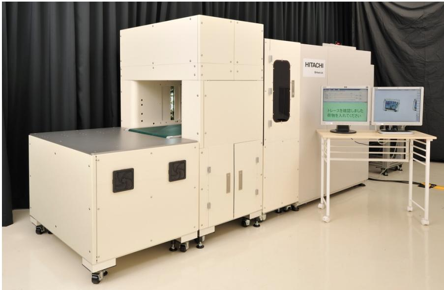
Prototype explosives detection system for carry-on luggage
