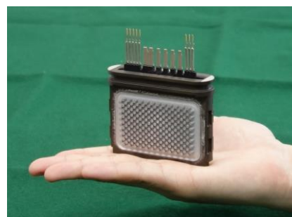
A compact and high-efficiency power module with double-sided cooling is built into Hitachi Automotive Systems' inverter
